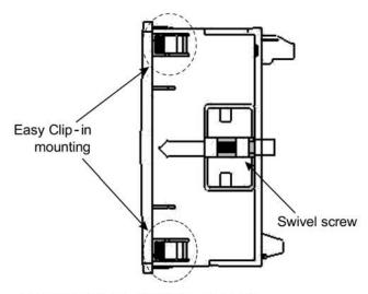
Panel Thickness: 1 - 3 mm for self clicking, 1 - 6 mm for swivel screws.
