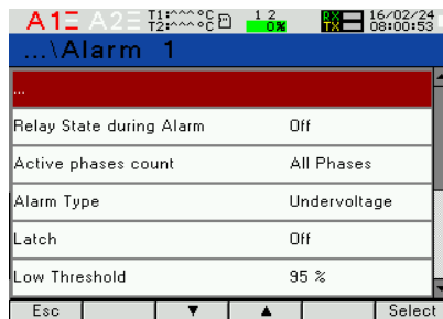
Fig. 23. Screens of Alarms mode
