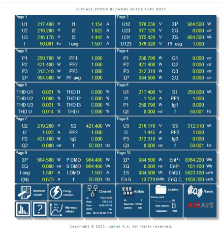
Fig. 36. View of the meter website
