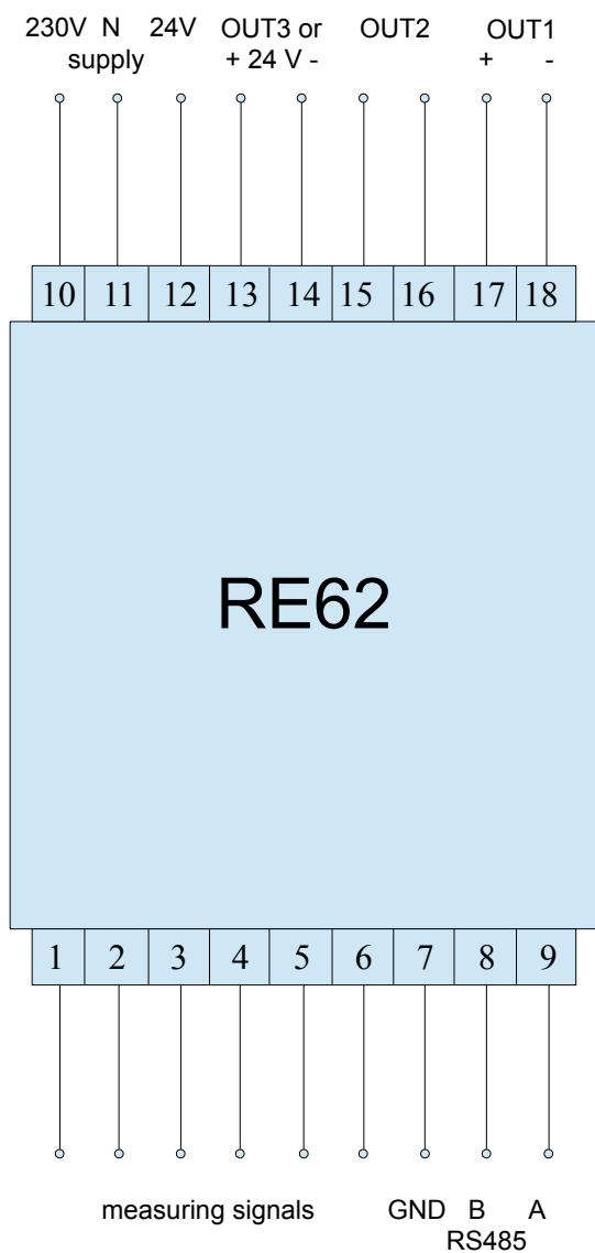
Figure 3. RE62 controller electrical connections
