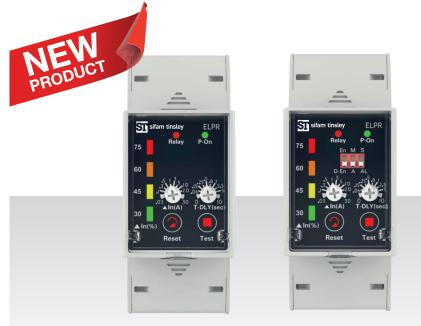
Sifam Tinsley ELPR is earth leakage relay (ELR), a protection device to be used in electrical installations against electric shock and / or damage to equipment caused by punctured or weak insulations or contact to live parts. Instrument operates by monitoring the earth leakage current through CBCT and disconnecting the circuit in case of hazardous levels of earth leakage currents. Sifam Tinsley ELPR is available in two versions, Smart and Smart+
