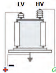
LV winding (with 3 phases short) to ground with HV winding guarded
