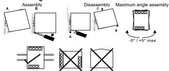
Other models / modules must have a minimum vertical and horizontal distance of 10 cm to this power supply in order to guarantee sufficient auto convection. Depending on the ambient temperature and load of the device, the temperature of the housing can become very high!
