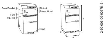
are single output, IP20, have Mounting DIN Rail IEC 60715/TH35. Class 2 isolation for FLEX - e 6024A and Class 1 for FLEX - e 24Volt (With Earth terminal) devices
