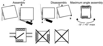
Other models / modules must have a minimum vertical and horizontal distance of 10 cm to this power supply in order to guarantee sufficient auto Addistance of 10 cm to this power supply in order to guarance sumound data
