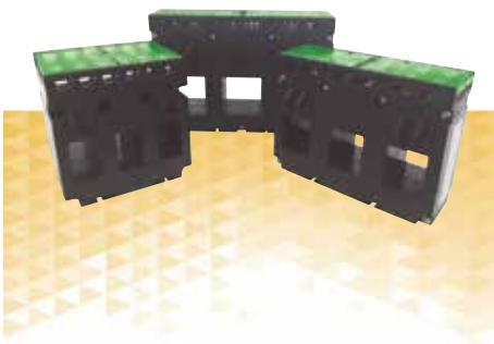
Three phase measuring current transformers suitable for primary ranges from 60A to 630A with 5A secondary. Allowing installations directly next to the moulded case circuit breakers for greater speed of installation and optimisation of space. Applicable to MCCB such as Manufacturers: ABB, Hager, Dorman Smith, Schneider, Terasaki, Merlin Gerin, Chint, Legrand plus many more.
