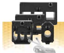
Omega single and 3 Phase RJ12 Current Transformers suitable for primary ranges from 50 to 600A with 100mA secondaries, with RJ12 connection for simple and easy error free installation.
