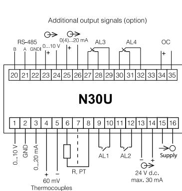
Fig. 1 Description of signals on connection strips.
