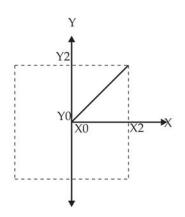
X0 = Start value of input X2 = End value of input=UN/IN UN = Nominal input voltage
