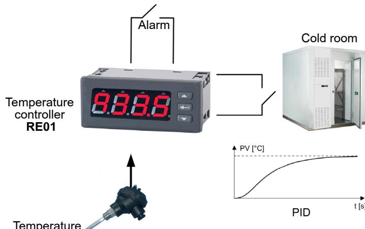
Automatic control of the cold room using the PID algorithm with autotuning function.
