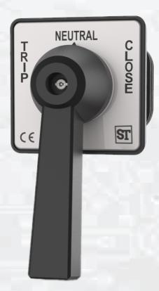
**EPSILON Cam TNC Series** TNC switch is a three position switch, when it is in close position it put the circuit breaker in operation by energizing the closing coil and when it is in trip position it will trip the circuit by energising the trip coil in circuit breaker.
