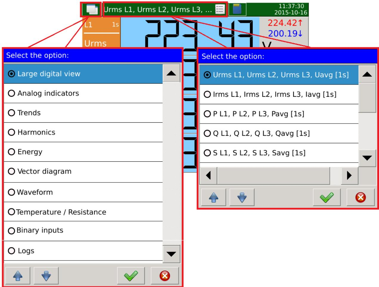
**Fig. 30. Navigation - switching views and screen.**
