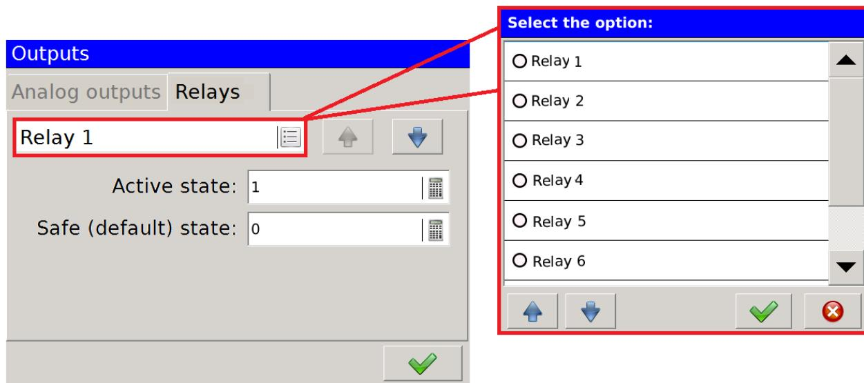
Fig. 138. Outputs - relays.
