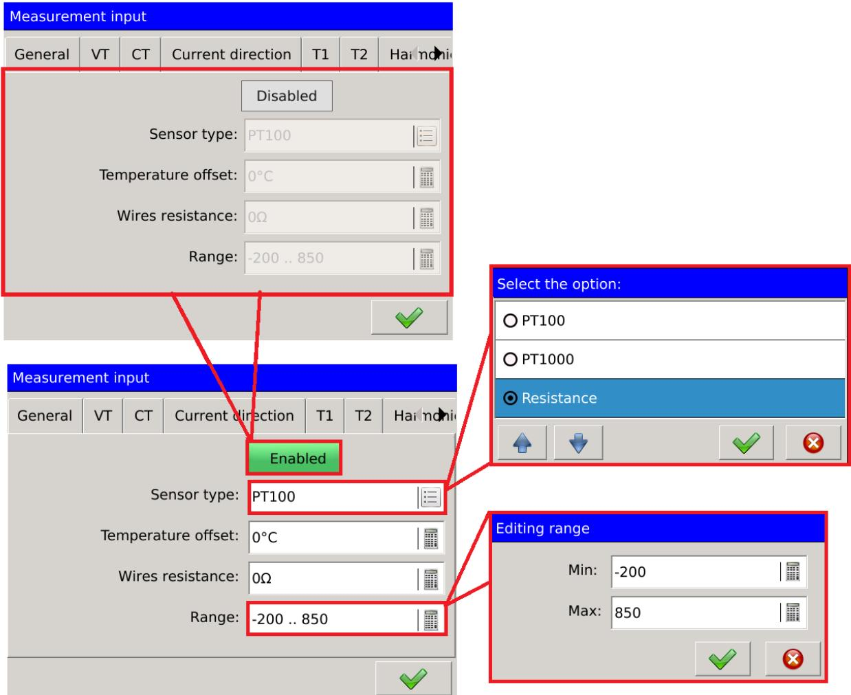
Fig. 111. Measurement input - temperature/resistance.
