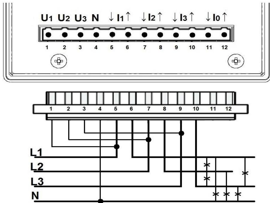
Fig. 5. Diagram - 4-wire network.
