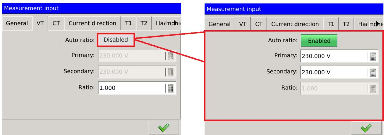
Fig. 108. Measurement input - voltage transformer ratio.
