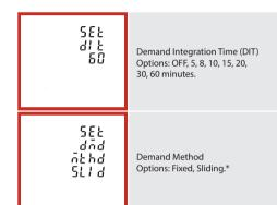
\* The Demand Method can be configued as follows: Sliding = 0~60 minutes, 1~61 minutes, 2~62 minutes etc Fixed = 0~60 minutes, 60~120 minutes, 120~180 minutes etc
