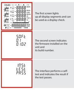
\*After a short delay, the screen will display active energy measurements.
