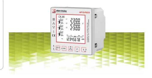
**Sifam Tinsleys AP15-P5CO** is a new generation modern design power monitor that will measure and display electrical power quality parameters. It has been engineered to cover most applications (Single Phase and Three Phase networks / Built in Pulsed and RS485 Modbus / Import and Export kWh), replacing the need for several different models of this power meter.
