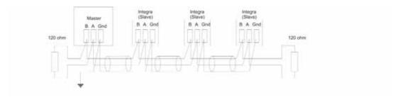
There must be no more than two wires connected to each terminal, this ensures that a "Daisy Chain or "straight line" configuration is used. A "Star" or a network with "Stubs (Tees)" is not recommended as reflections within the cable may result in data corruption.
