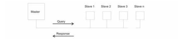
In the Modbus™ Protocol the master can address individual slaves, or, using a special "Broadcast" address, can initiate a broadcast message to all slaves. The AP15-P5CO digital power measurement meter does not support the broadcast address.
