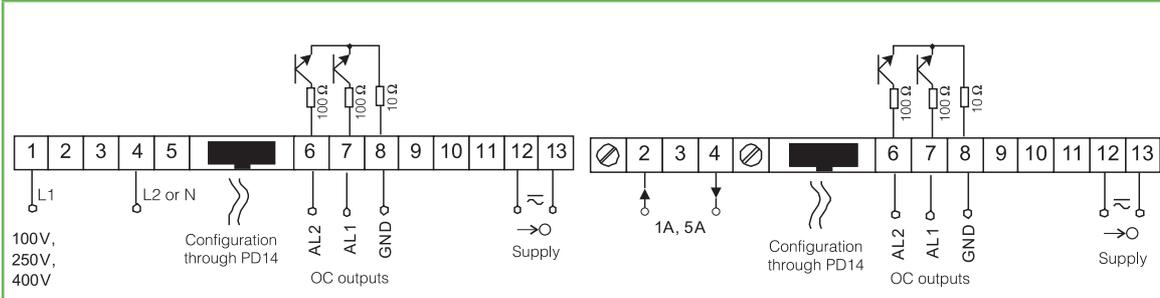
Fig. 1 Electrical connections of the N20Z meter with the measurement of voltage and frequency.
