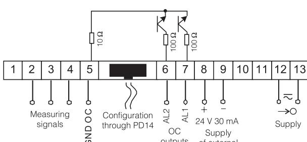
Fig. 1 Electrical connections of N20 meter.
