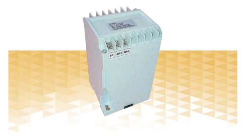
Omega Summation current transformers are designed to summarize several synchronous Alternating Currents of equal phase relation with any angle of phase difference, They are used to add secondary currents of several main C.T.'S in order to measure with one CT only. The output current again constitutes a standardized quantity. That means the primary currents are not only added but also divided by the number of inputs.
