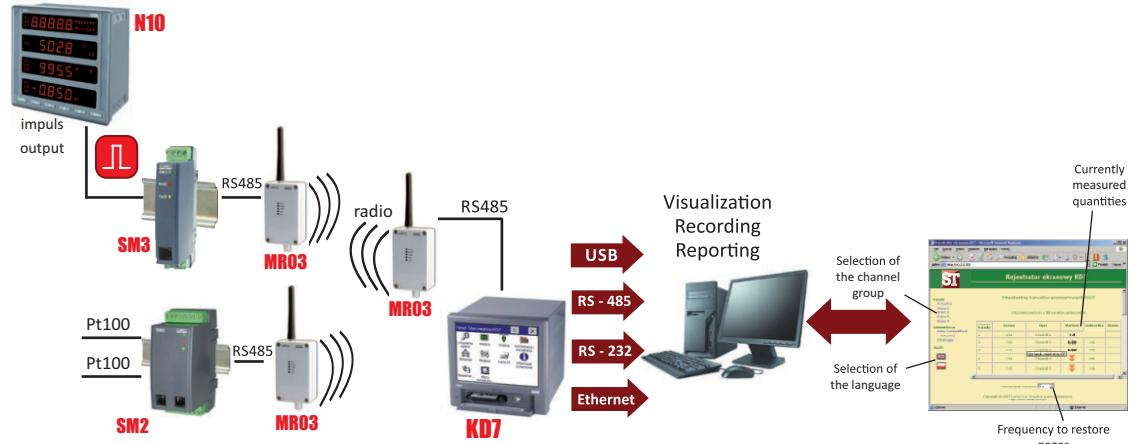
System of measurement, control and recording of temperature and energy with wireless communication.
